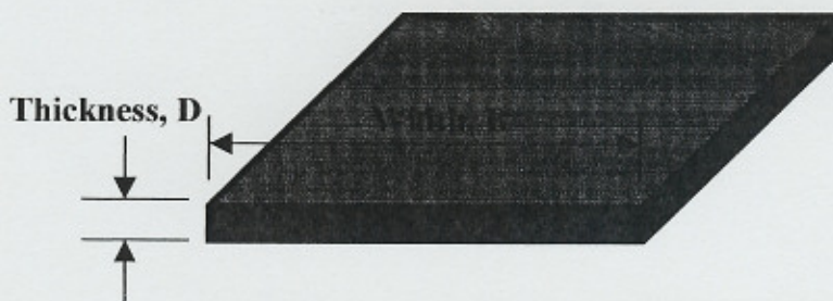
Fig 8 Factors used to calculate stiffness of solid rotomoulded part
